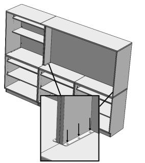
8. If monitor hutch is not attached to other hutches, additional screws need to be used to attach backside of hutch to base cabinet. Use a 9/64" drill bit to drill holes into the base cabinet through the holes in the hutch.
