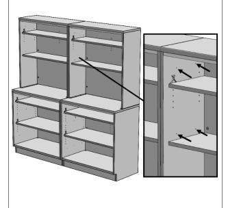
**4.** Insert supplied connector bolts through drilled holes to connect hutches.
