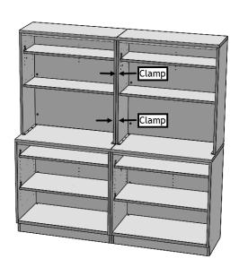
3. Locate partially predrilled holes on end panels. Use a 5/16" drill bit to drill (4) holes through end panels of hutches to be joined.
