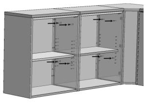
**4.** For corner cabinets, drill through partially predrilled holes into corner end panels. Install (4) #10 X 1.25" wood screws through holes into each adjoining cabinet end panel (8 total.)
