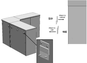
3. All hanging cabinets are required to be connected at the end panels. (8) #10 x 1.25" wood screws are included for each corner cabinet. All other cabinets include (4) connector bolts per end panel.
