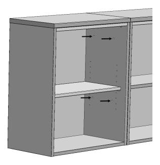
**6.** Place connector bolt through drilled holes. Use a Philips screwdriver to tighten as needed. Repeat for the remaining attachment points.
