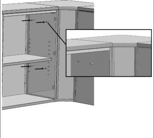
**5.** For all other cabinets, use a 5/16" drill bit to drill out holes for connector bolts at provided partially predrilled holes. There are (4) per end panel.
