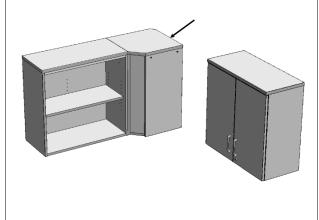
2. Attach brackets into wall studs using the included screws, and hang cabinets on brackets. Next, attach each cabinet to the wall with at least one screw to prevent dislodging. If the included brackets will not work with building construction, use another approved hanging method to mount cabinets securely to the wall per local codes and regulations.
