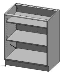
**2.** Extend front levelers on all additional cabinets and slide into place next to first cabinet. Adjust levelers as needed to align cabinets.
