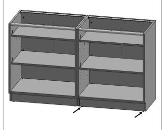
**3.** After aligning cabinets, reach under the top and push the quick connect clip until it engages with the slot on the adjacent cabinet.
