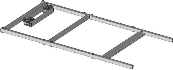
**2.** Move the feet into position as shown and insert (2) star locking washers and (2) ¼-20 fasteners for each foot. Tighten to a torque of 75-80 in-lb.
