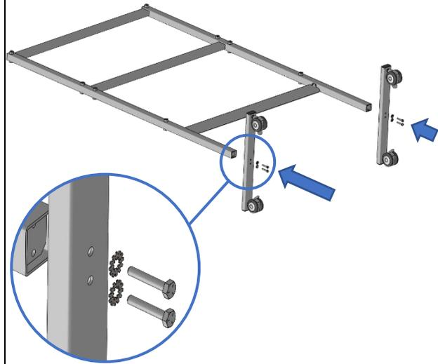
**3.** Rotate the tray 90 degrees clockwise and install one #10 screw at each end. Tighten to a torque of 30.0-35.0 in-lb.
