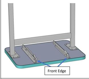
2. (If your product has pilot holes, skip to step 3.) Align the rails as shown below and mark the hole locations. Drill (3) 0.125" diameter by 0.500" deep holes for each rail.
