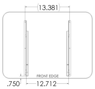
**3.** Attach the rails to the worksurface using (3) #8 X 0.625" screws for each rail. Tighten to a torque of 30-35 in-lb. (Frame removed for clarity.)
