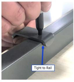
3. Attach the bag hook to the rail using the supplied self-drilling screw. Position the screw straight as you drive it in and stop once the screw head is tight to the bag hook. Do not overtighten the screw. Overtightening the screw will cause the threads to fail and the attachment will be
