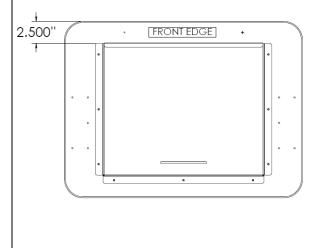
3. Attach the book box to the worksurface using (9) #8 X 0.625" screws. Tighten to a torque of 30-35 in-lb. (Frame hidden for clarity.)
