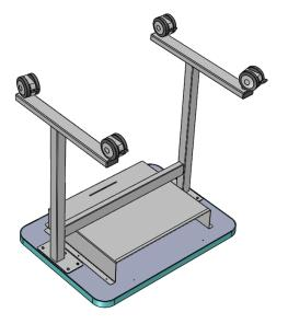
2. (If your product has pilot holes, skip to step 3.) Align the book box as shown below and mark the hole locations. Drill (9) 0.125" diameter by 0.500" deep holes.
