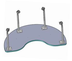
2. Place the tube into position on the worksurface, lining up the screw holes. Dimples should face away from the
