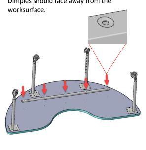
**3.** Attach the tube support to the worksurface using (4 or 5, depending on the table size) #10 X 1.5" screws. Tighten to a torque of 30-35 in-lb
