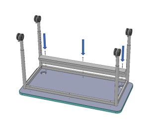
3. Place the wire trough into position on the bottom of the worksurface. Insert (3) #10 x .500" screws through the holes in the trough and into the pilot holes in the worksurface. Tighten to a torque of 30 to 35 in-lb.
