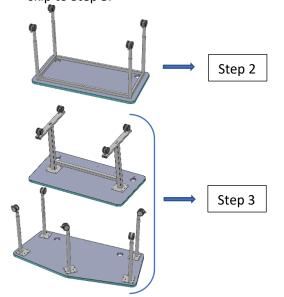
2. Place the wire trough into position on the steel frame. Insert (3) #10 x 2.000" screws through the holes in the trough and the steel frame, and into the pilot holes in the worksurface. Tighten to a torque of 30 to 35 in-lb.
