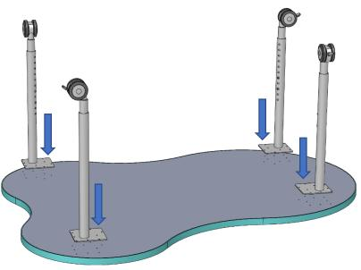
2. Insert (9) #10 x .875" screws through the holes in the top plate of each leg and into the pilot holes in the worksurface. Tighten to a torque of 30 to 35 in-lb.
