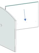
3. Locate the worksurface. Attach the worksurface to the end/intermediate panels. Note the relief cutouts on the bottom of the worksurface near each of the modular clips. Slide the worksurface between the end/intermediate panels until the relief cutouts align with the shoulder screws. Lower the worksurface and slide toward the back panel to engage the shoulder screws. Use the rubber mallet to properly seat the modular clips onto the shoulder screws.
