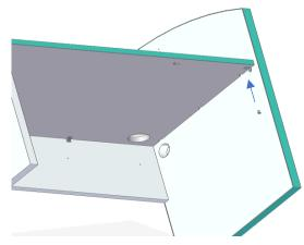
**6.** Locate the wire management trough. Align the holes in the wire management trough to the holes in the back panel below the worksurface. Attach by using #8 x 5/8 screws .
